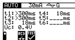
Figure 5.23: Step 4 RCD auto test results
