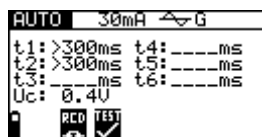
Figure 5.21: Step 2 RCD auto test results
