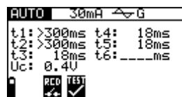
Figure 5.24: Step 5 RCD auto test results
