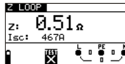
Figure 5.28: Example of loop impedance measurement results
