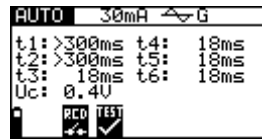
Figure 5.25: Step 6 RCD auto test results
