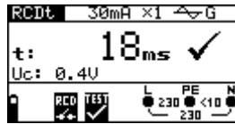
Figure 5.16: Example of trip-out time measurement results
