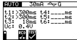
Figure 5.22: Step 3 RCD auto test results
