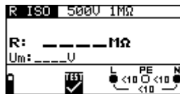
Figure 5.1: Insulation resistance measurement menu
