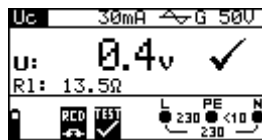
Figure 5.14: Example of contact voltage measurement results
