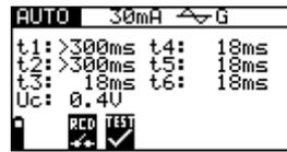
Figure 5.25: Step 6 RCD auto test results
