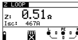
Figure 5.28: Example of loop impedance measurement results
