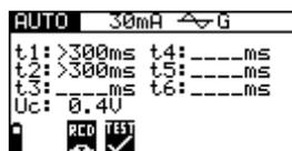
Figure 5.21: Step 2 RCD auto test results
