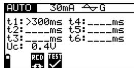
Figure 5.20: Step 1 RCD autotest results
