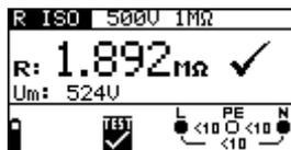
Figure 5.3: Example of insulation resistance measurement results
