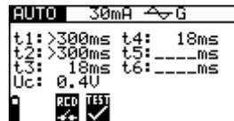
Figure 5.23: Step 4 RCD auto test results
