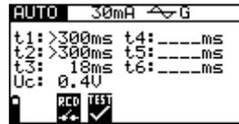
Figure 5.22: Step 3 RCD auto test results
