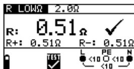
Figure 5.7: Example of LowΩ resistance measurement results
