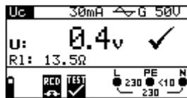
Figure 5.14: Example of contact voltage measurement results
