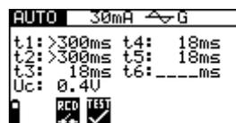
Figure 5.24: Step 5 RCD auto test results
