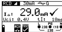
Figure 5.18: Example of trip-out current measurement result
