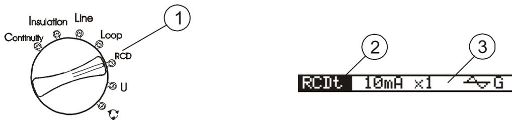
Figure 4.2: Function selector switch and belonging parameter line
