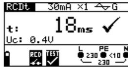
Figure 5.16: Example of trip-out time measurement results
