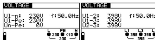
Figure 5.39: Examples of voltage and frequency measurements
