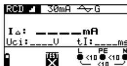
Figure 5.17: Trip-out current measurement menu
