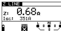
Figure 5.33: Example of line impedance measurement results
