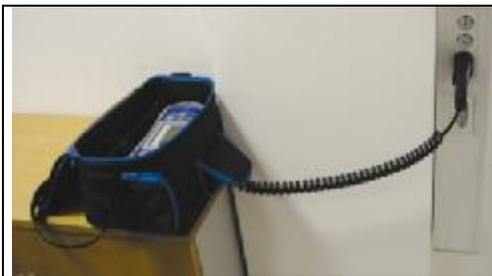
The instrument can be used even placed in soft carrying bag – test cable connected to the instrument through the front aperture.
