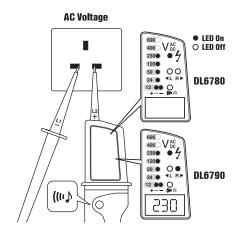
Always hold the test probes by the handles behind the finger guards.. Observe the safety notices at all times.
