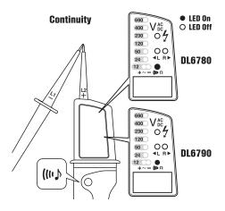
Note: The continuity test is only possible when batteries are installed and in good condition
