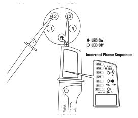
Connect test probe L2 to the supposed phase 3 and test probe L1 to the supposed phase 2. If the R LED illuminates the phases are in the correct sequence 2 to 3. Connect test probe L2 to the supposed phase 1 and the test probe L1 to the supposed phase 3. If the R LED illuminates the phases are in the correct sequence 3 to 1.
