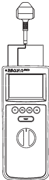
Figure 6 Mains Voltage/RCD/Earth Loop Impedance /Line Impedance Measurement
