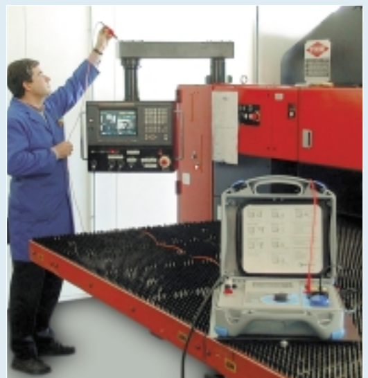
Complete testing of safety on machines (at initial installation or on periodic basis)
