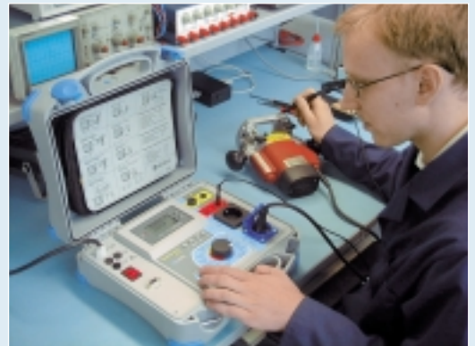
Final test on a portable appliance in a service workshop
