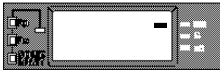
Fig. 3 Low battery voltage indication
